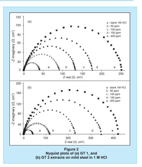
The usefulness of these data permits the analysis of the alternating current (AC) impedance data, which are based on the modelling a corrosion process by an electrical circuit (Hussin & Kassim, 2010).
