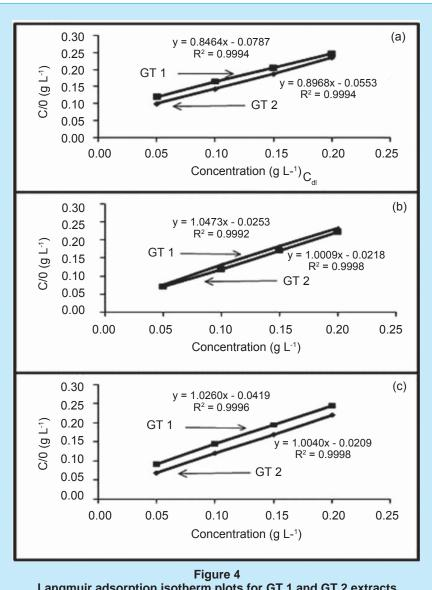
Langmuir adsorption isotherm plots for GT 1 and GT 2 extracts on the mild steel surface from (a) weight loss, (b) potentiodynamic and (C) EIS measurement far the most popular technique for analysing tea catechins. Wang et al. (2000) reported on the use of methanol/ water and acetonitrile/water as mobile phase for the catechin analysis. The catechin monomers and caffeine were separated in about 40
