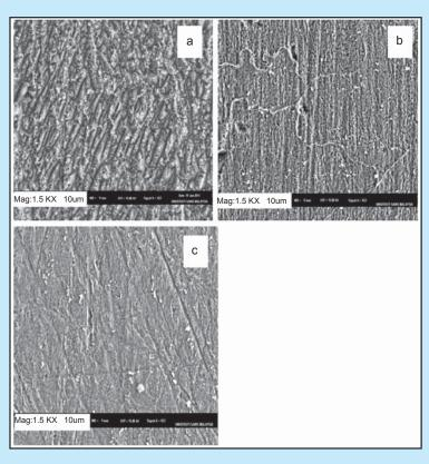
Figure 8 SEM images of mild steel in 1M HCl medium (a) absence of inhibitor (b) GT 1, and (c) GT 2 extracts
