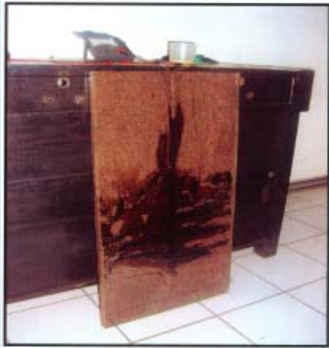
Figure 1 A physical model comprises granite crack containing crude oil simulating fracture basement reservoir
