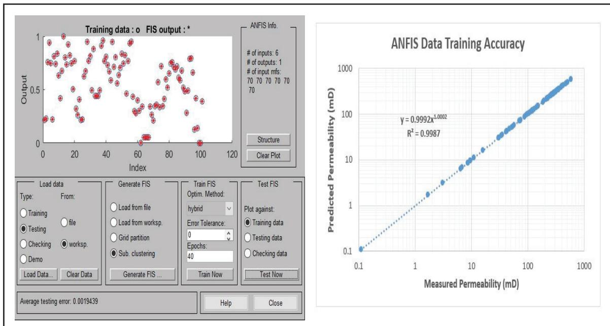
Figure 6 Training data result before denormalization (Left) and After denormalization (Right).
