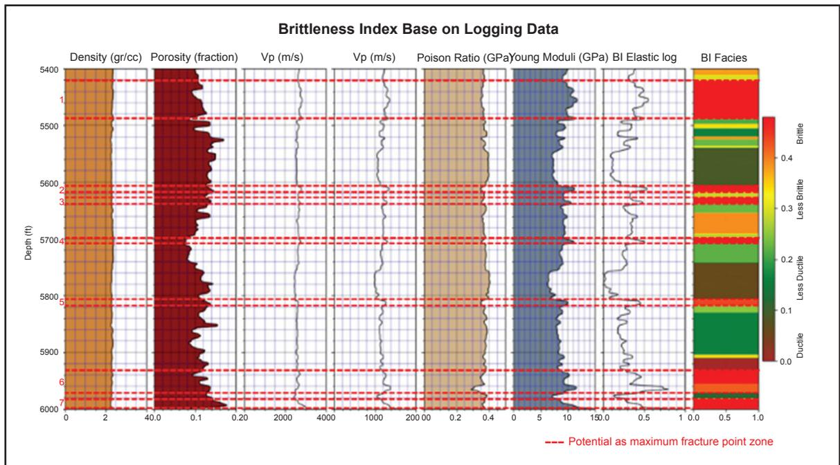
Figure 3 Brittleness Index interpretation based on elastic properties of data logs with maximum fracturing point location.
