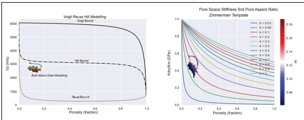
Figure 4 Voigt Reuss Hill modeling (Mavko, Mukerji, & Dvorkin, 2020), (b) Pore aspect ratio distribution using Zimmerman's constant pore space stiffness (Russell & Smith, 2007).
