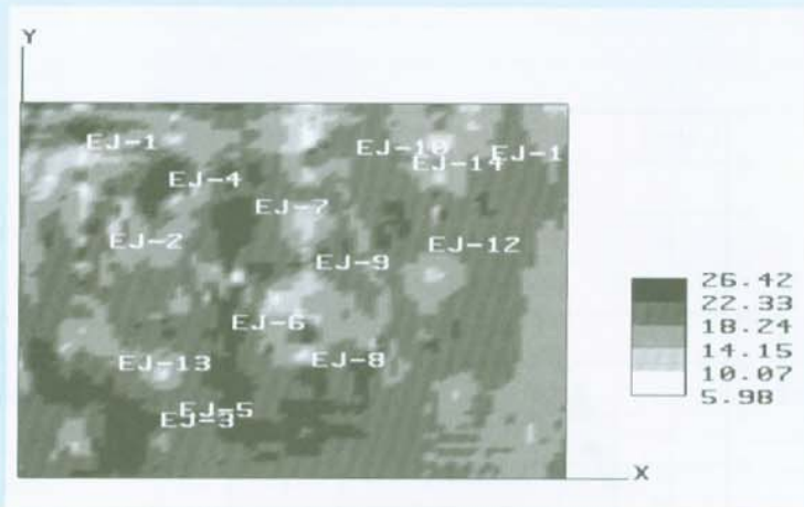
Figure 12 Porosity lateral distribution for the top 10 microseconds interval of EJ reservoir
