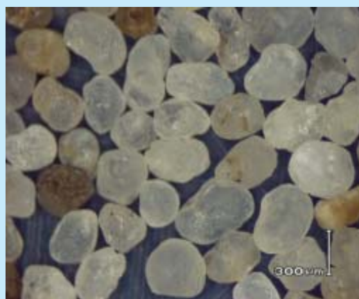
Figure 5 Grain shape processing sand with size 20/40 of Location I
