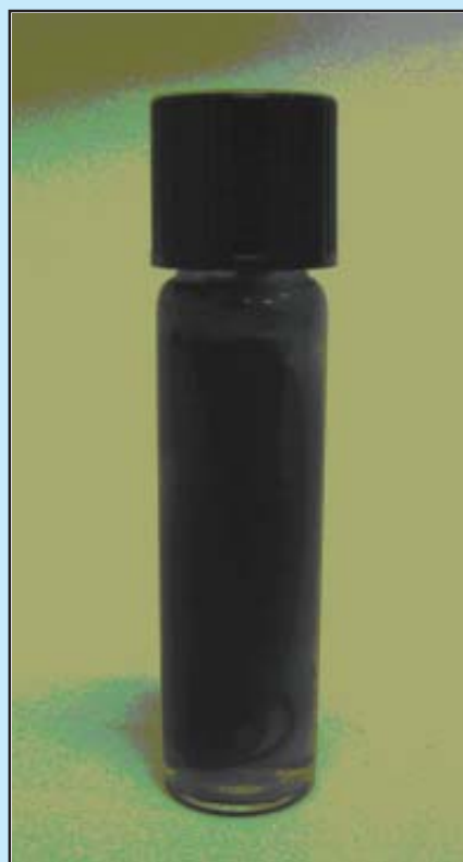
Figure 2.1 A sample contains sulfate reducing bacteria with black colour tube appearance
