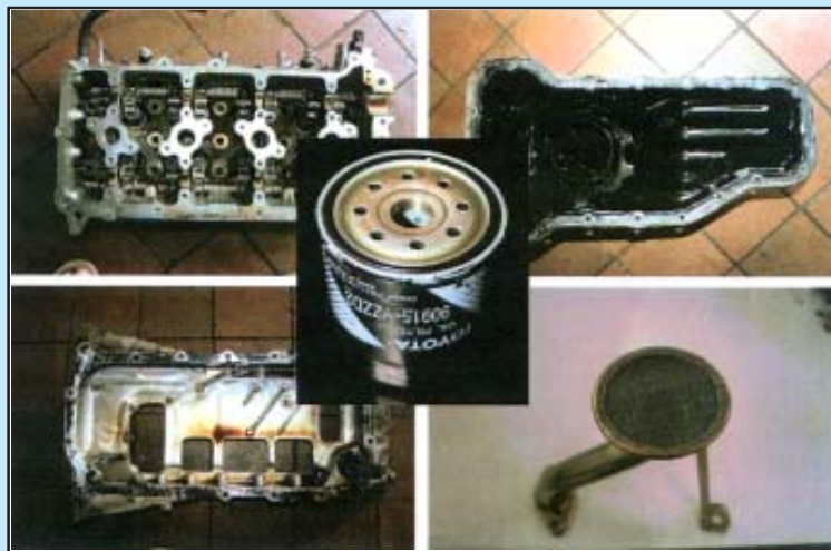
Figure 10 Sludge and varnish formation
