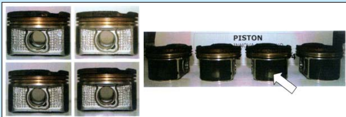
Figure 4 Piston condition (Skirt Varnish)
