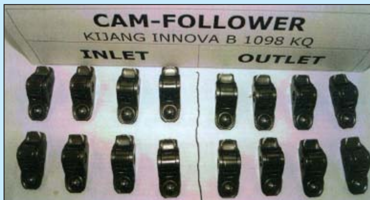
Figure 7 Camshaft follower condition after road-test
