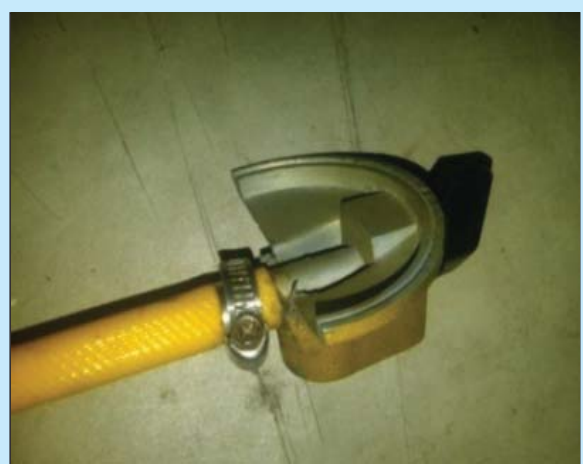
Figure 2 Regulator for connecting to the LPG storage
