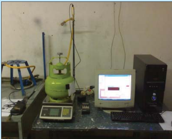
Figure 1 Installation of instrument at gas leak research
