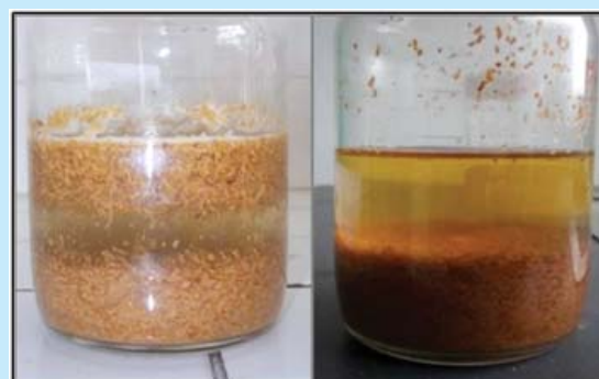
Figure 3 Rice husk pre- (left) and post- (right) dilute acid pretreatment
