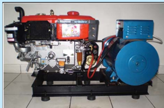
Figure 1 Diesel engine generator 5 KVA
