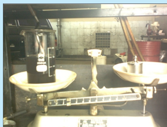
Figure 5 Measurement of fuel consumption time-based method
