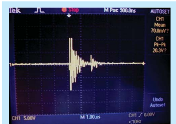
Figure 9 The signal on tranducer with water medium
