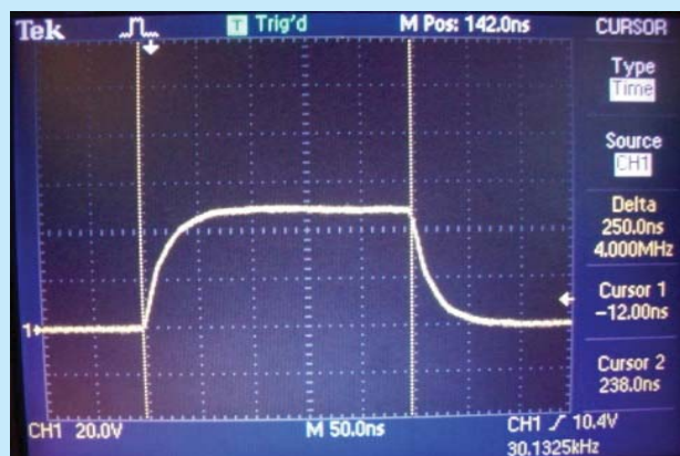
Figure 8 The form of excitation pulse ultrasonic generation on pulse as wide as 250 ns
