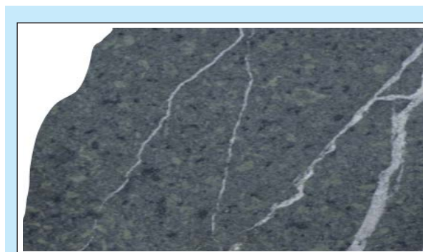
Figure 3 Fracture photograph of slabing core taken from basement rock
