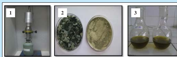
Figure 2 Cell disruption using ultrasonic; (1) ultrasonic equipment; (2) dried algae and (3) crude alga oil
