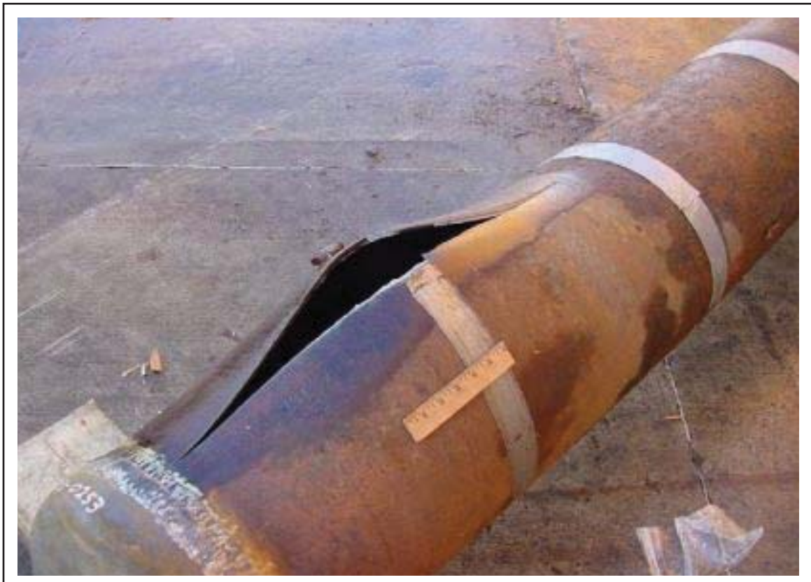
Figure 2 Casing when burst rating is exceeded.
