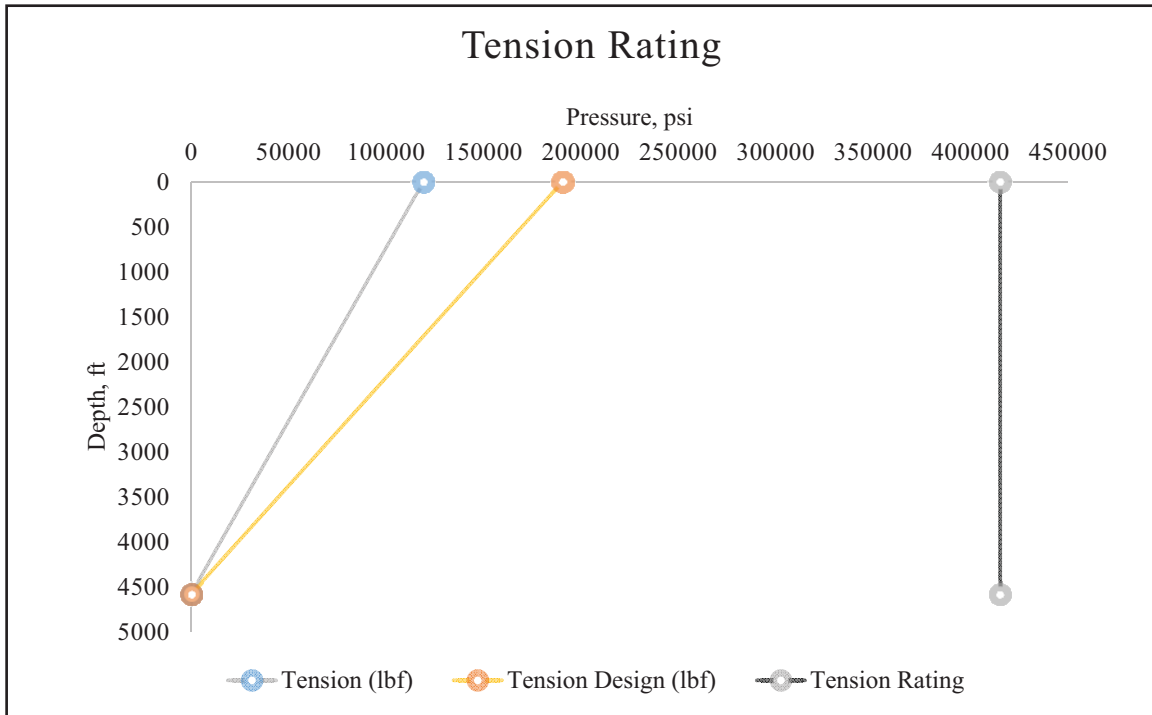
Figure 14 Tension rating of production casing.
