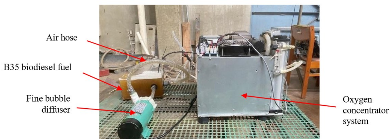
Figure 1. Experimental setup for ultrafine bubble (UFB) injection into B35 biodiesel fuel.
