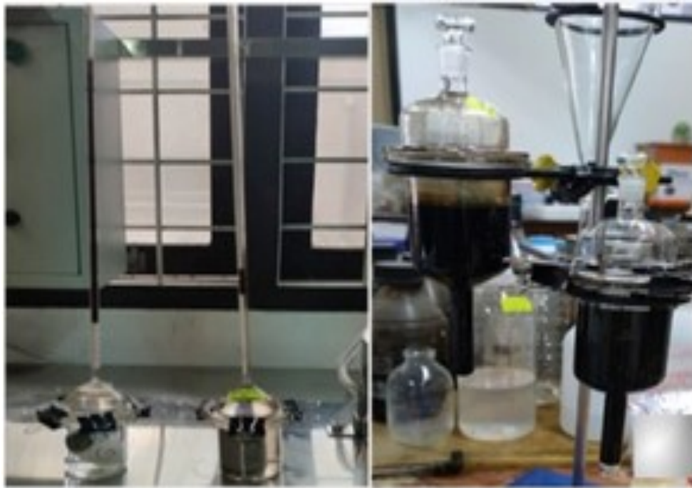
Figure 6. Amott cell measurement for wettability index
