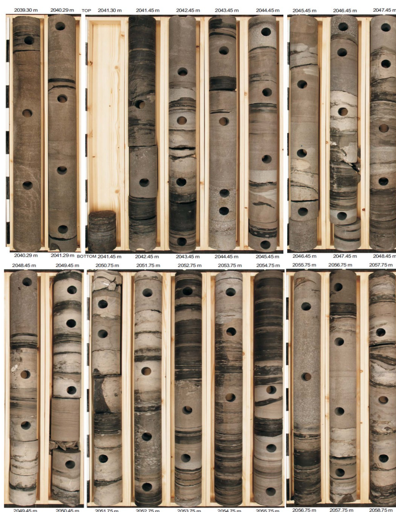
Figure 7. Large-Scale Cores for HABBAN 28.
