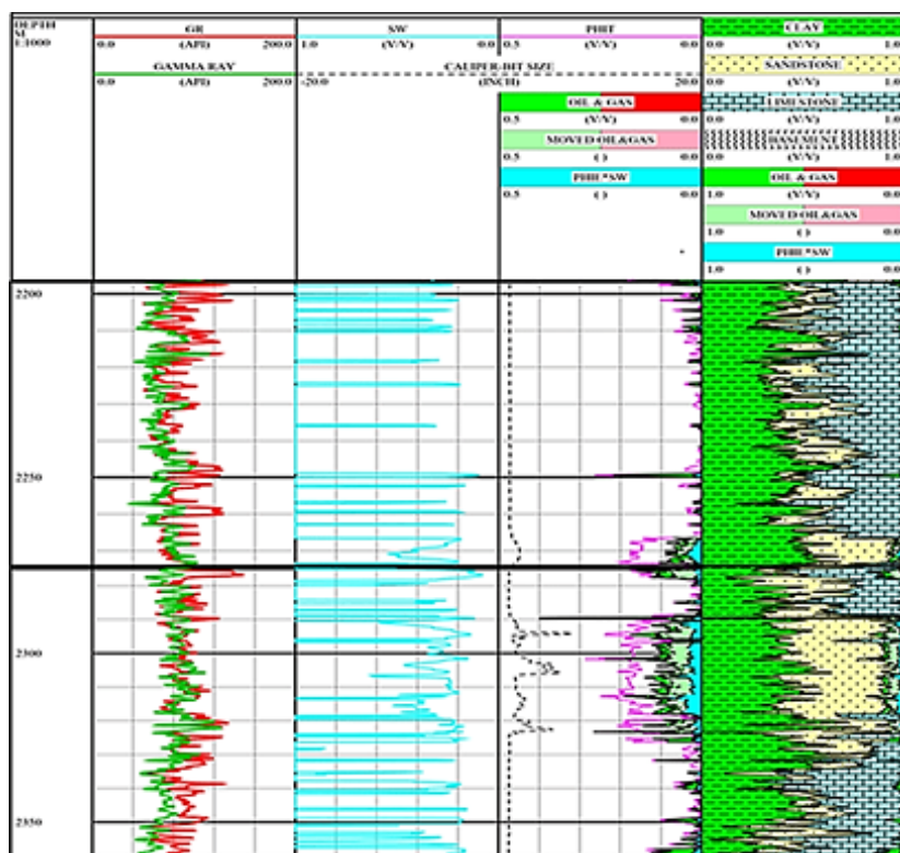
Figure 15. Petrophysical log interpretation of test interval in lower Lam Member of NIL-1 well showing better reservoir quality and movable oil saturation.
