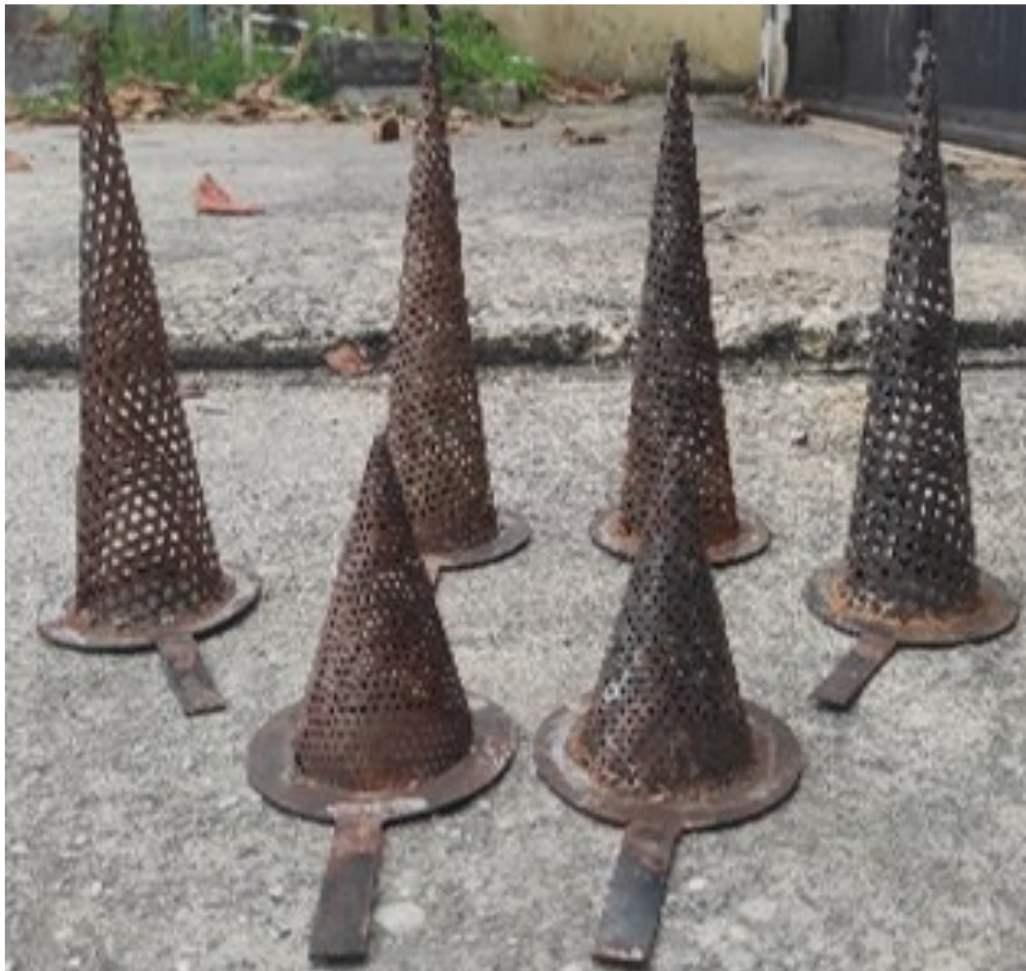
Figure 3. Strainer geometry with the hole pattern and manufacturing results
