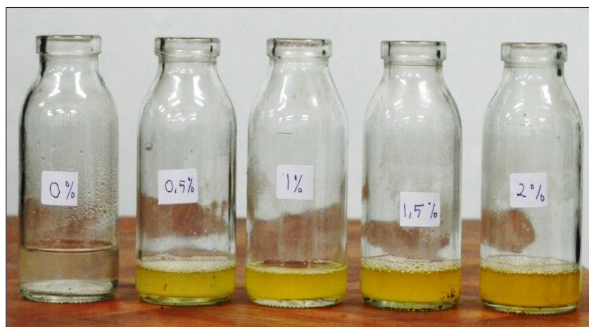
Figure 1. Rhamnolipids solution samples at different concentrations prepared prior to IFT and viscosity measurements
