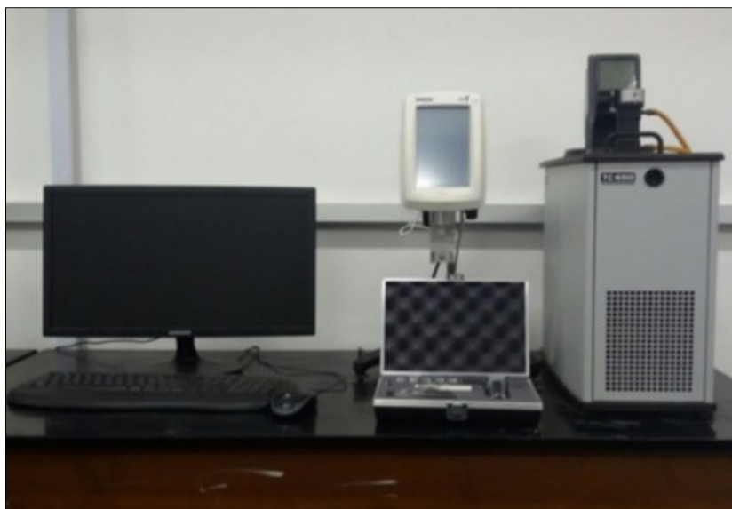
Figure 3. Brookfield DV3T rotational viscometer used to measure emulsion viscosity with instrument speed range is 0.01–250RPM
