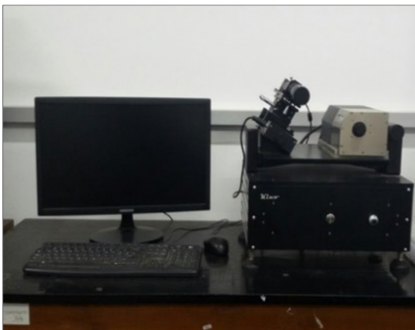
Figure 2. Spinning drop interfacial tensiometer used for oil-brine IFT measurements, with \pm 3 RPM control accuracy
