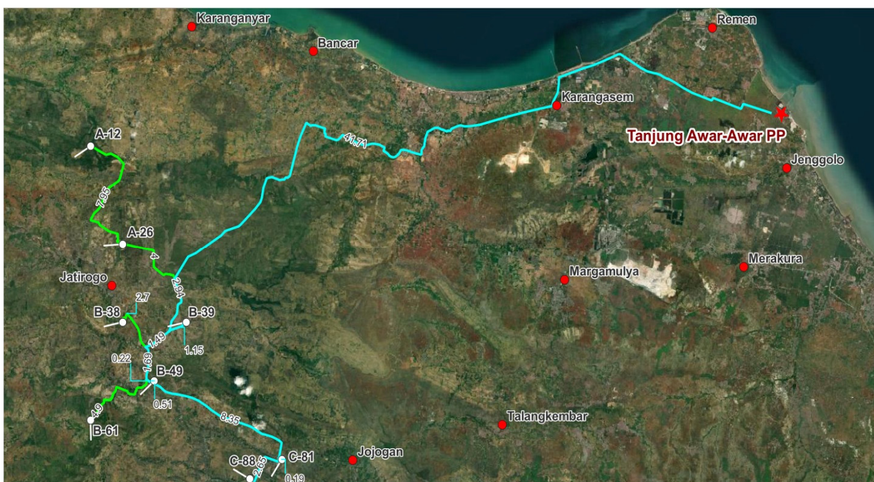
Figure 8. Optimized CO_2 transmission pipeline from the Tanjung Awar-awar power plant to the storage site. The line with cyan color represents Scenario A, whereas additional lines for additional wells needed in Scenario B are in green.
