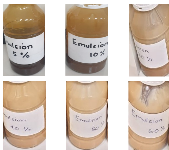
Figure 2. Photographs of W/O emulsions prepared from used lubricants and brine at water fractions of 5–60 vol%. Increasing the water fraction changes the emulsion colour from dark to light brown, while all samples remain visually homogeneous and show no macroscopic phase separation
