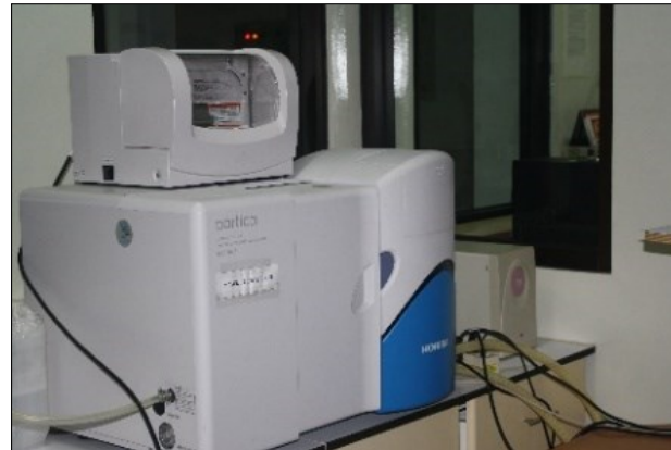
Figure 5. HORIBA laser scattering particle size distribution analyzer LA-950 (manual book)
