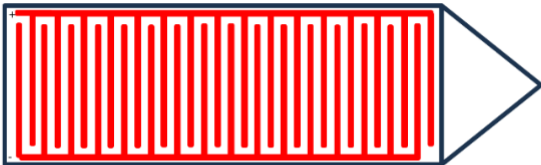
Figure 2. IDC Sensor design. The figure shows a planar interdigital capacitor (IDC) sensor, consisting of interleaved metal fingers that produce a fringing electric field.
