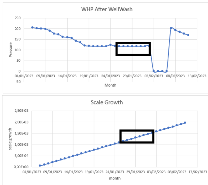
Figure 4. Temporal comparison between production performance and estimated calcite scaling growth following the well washing intervention. Production rate and scaling growth are shown as relative trends over time, illustrating short-term production recovery and subsequent decline.
