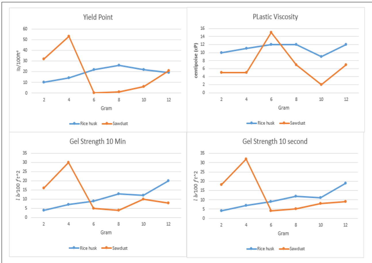
Figure 8. The effect of rice husk and sawdust addition on rheological properties of drilling Mud
