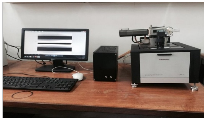
Figure.2 Spinning drop tensiometer series 500D
