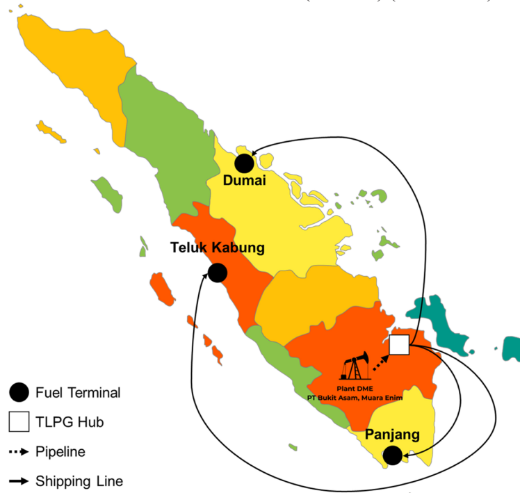
Figure 2. DME Distribution Pattern of Muara Enim Plant (Pertamina 2022; Kementerian Energi dan Sumber Daya Mineral Republik Indonesia 2021)
