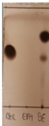
Figure 3. TLC Chromatogram of the Etherification Reaction of Oleyl Alcohol and EPH (Chromatogram TLC from the first step reaction shows Oleyl Alcohol reacted with EPH to form a new product, which is predicted to be Oleyl Gliscidyl Ether. This is proven by the difference in polarity, where OGE is more polar than OG.
