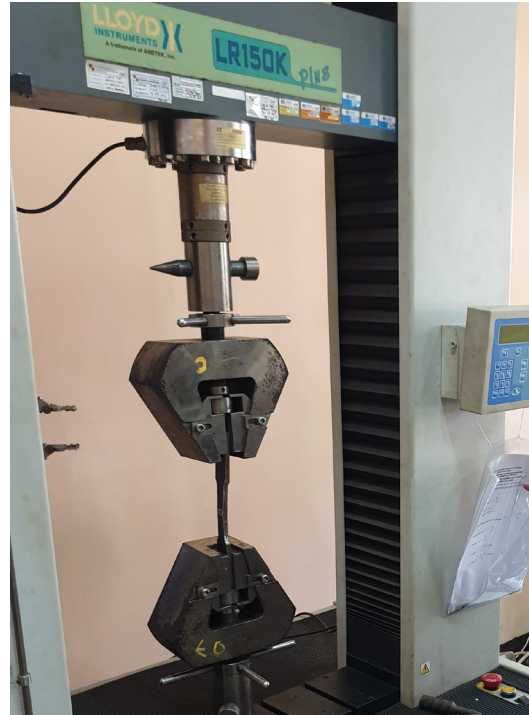
Figure 9. The tensile test process for the test specimen.
