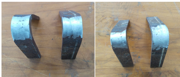
Figure 14. Face bend and root bend test result
