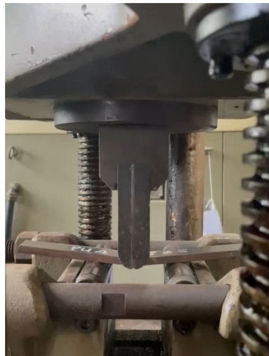
Figure 10. The bending test process for the test specimen
