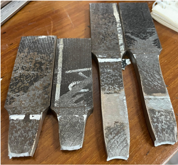
Figure 11. The tensile test results for the specimen
