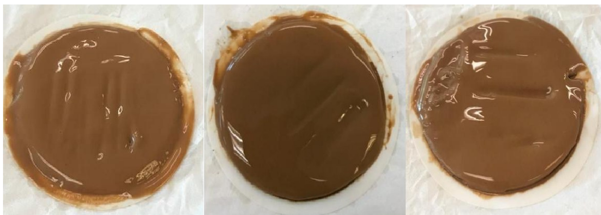
Figure 1. Mud cake thickness of sodium hydroxide contaminant used in this study.
