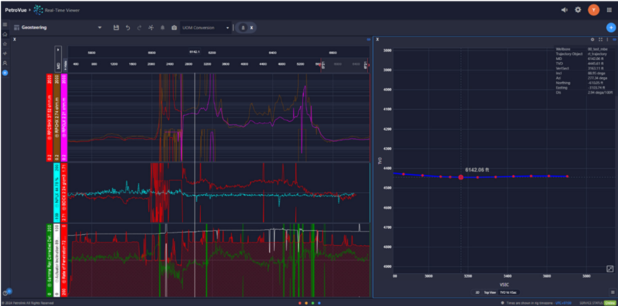
Figure 7. Trajectory station at 6142 ft was higher to keep the drillstring inside the reservoir zone.
