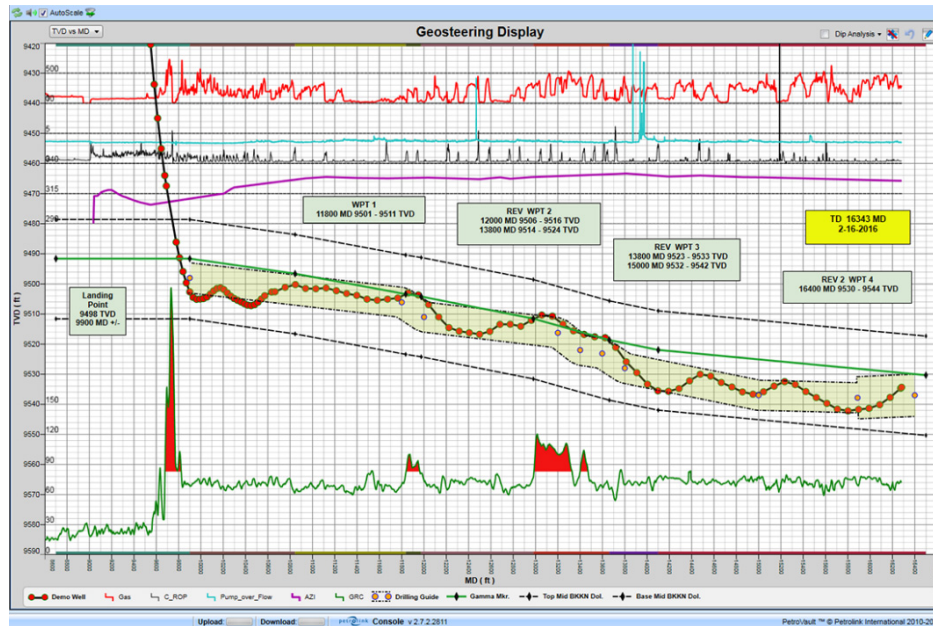
Figure 2. Geosteering display shows process involves drilling a precise path that aligns with the productive zone.
