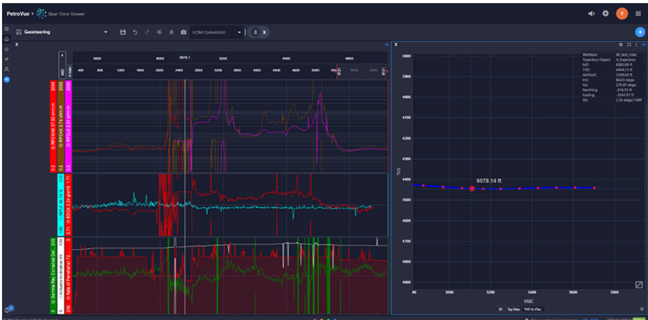
Figure 6. Trajectory station details at 6078.14 feet measured depth show around 88.03 degrees (before the alert was generated).
