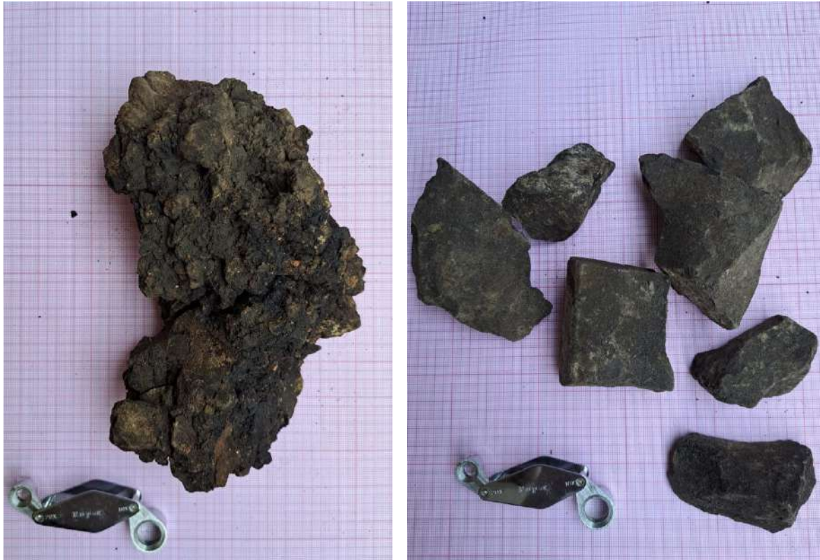
Figure 10 Appearances of (a) Lawele, and (b) Kabungka asphalt-containing rocks (collection of Research Center of Process Manufacturing Industry Technology)
