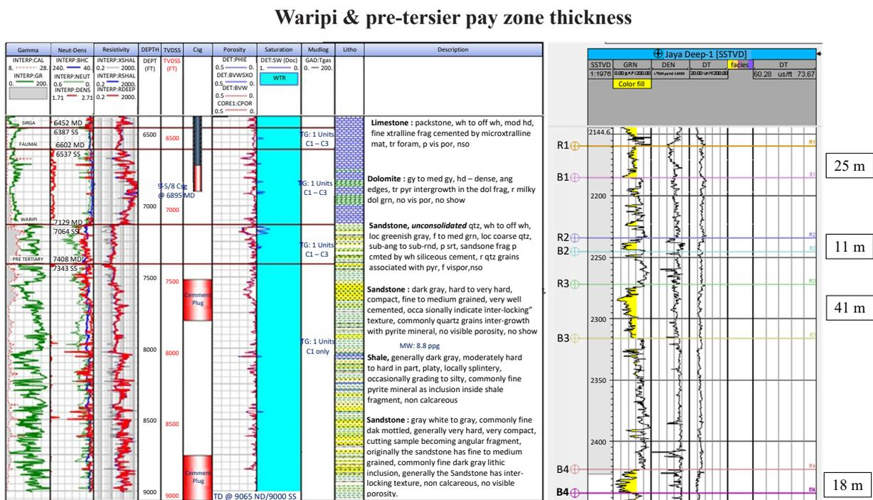
Figure 1 The geological and geophysical model of the reservoir pay zone thickness of kais, waripi, and pre-tertiary formation based on the jaya-deep-1 well are summarized using well log data.
