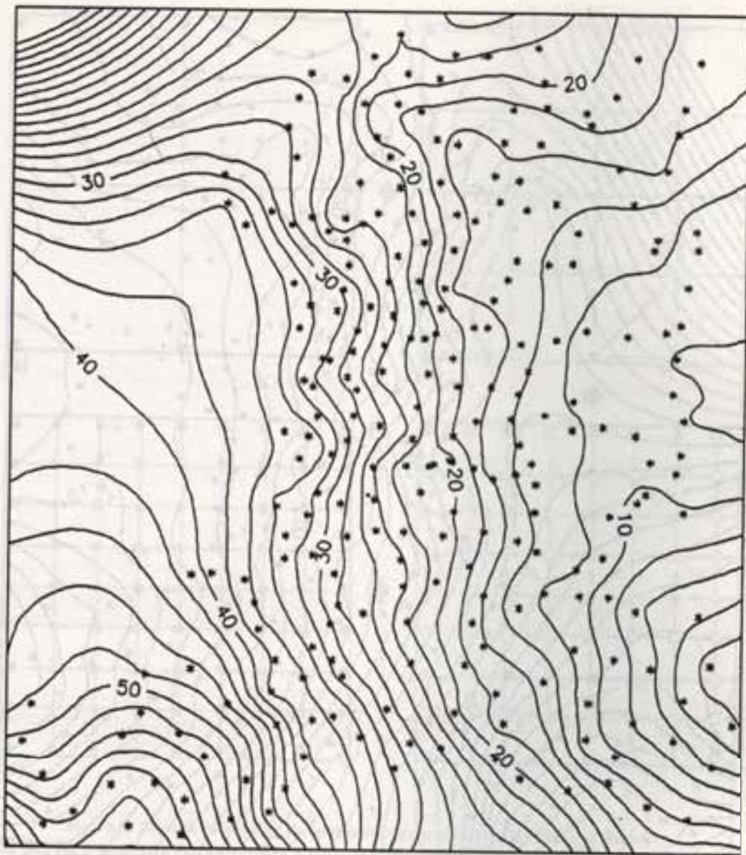
Figure 8. Gravity anomaly map, contoured based on a 49 by 43 grid interpolation result. Gravity stations are shown with stars; note that as the western and northwestern part of the area have no gravity stations, there is no judgment or control on those interpolation values.
