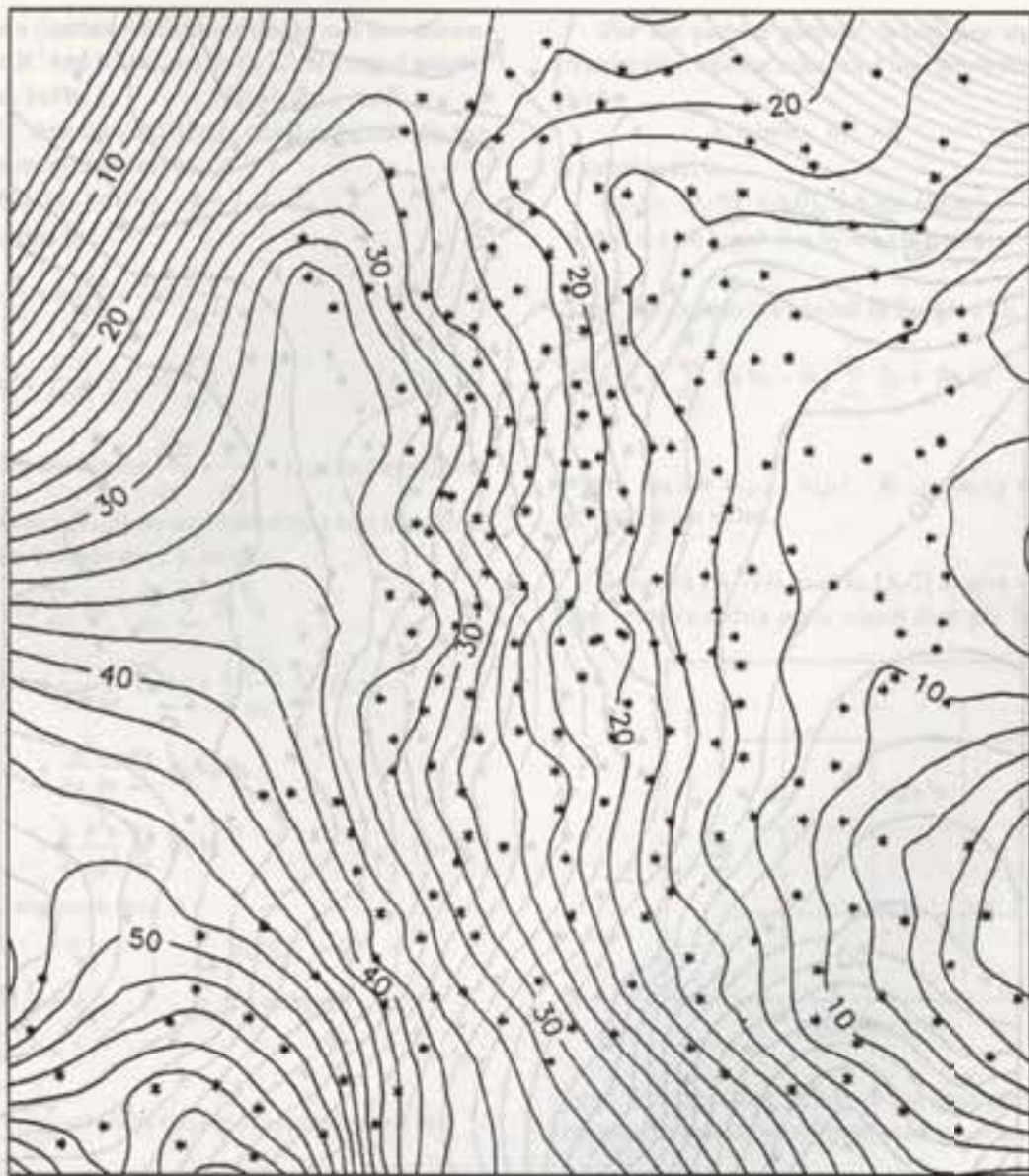
Figure 7. Gravity anomaly map, contoured based on a 33 by 29 grid interpolation result. Gravity stations are shown with stars; note that as the western and northwestern parts of the area have no gravity stations, there is no judgment or control on those interpolation values.
