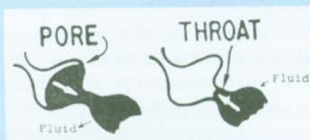
Figure 2 Model of fluid flowing across pore throat
