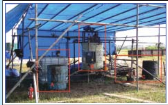
Gambar 1 Peralatan Pengolahan Tanah Tercemar Minyak dengan Teknik Bios (A) Washing Water Container , (B) Multi Purpose Reactor Unit & Control Panel , (C) Water & Oil Recovery Container
