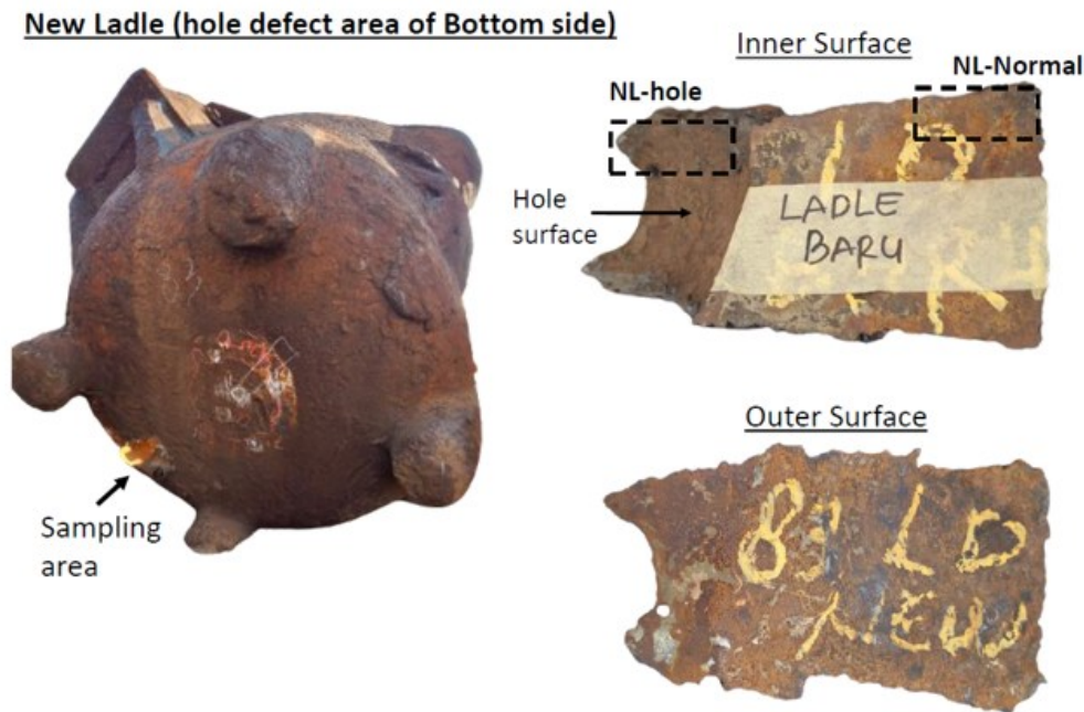
Figure 4. New ladle and leaking ladle sampling points
