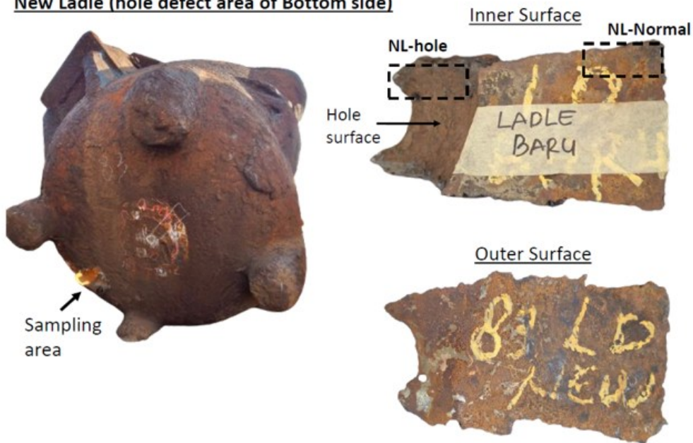
Figure 4. New ladle and leaking ladle sampling points
