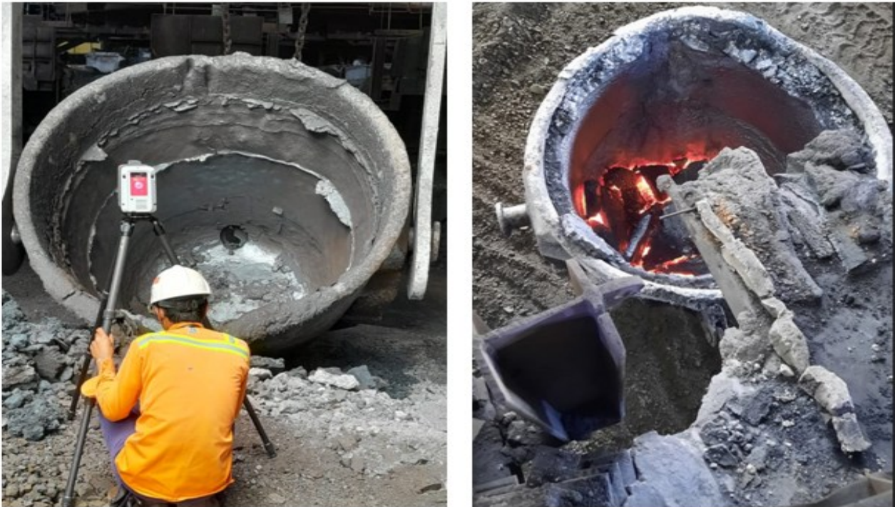
Figure 9. Converter slag deposit on the wall of a leaking ladle (left) with another ladle (right)
