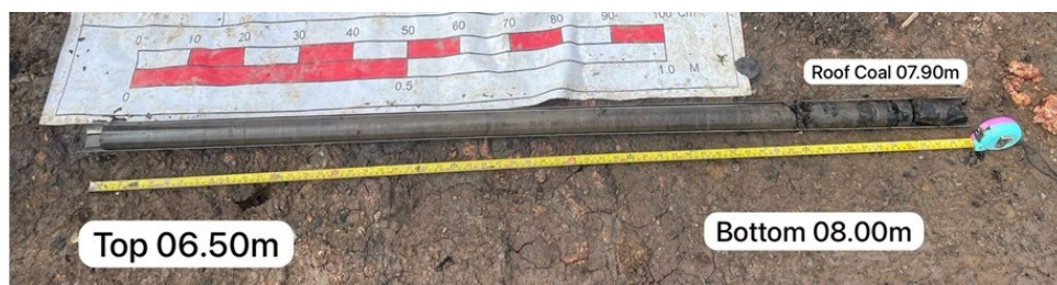
Figure 10. Appearance of claystone drill core in the field
